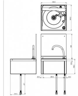
Knee operated wash hand basin is manufactured from stainless steel - satin polish finish, material thickness 0.9mm. Supplied complete with water spout positioned in rear right hand corner and 32mm waste outlet.
