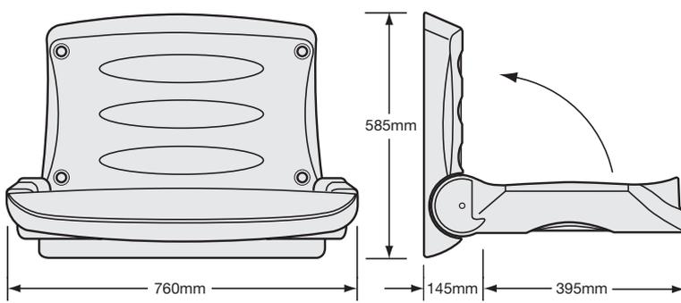
Suggested mounting height from the floor to the base of the unit is 730mm
