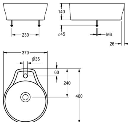
RONDAtop countertop basin, made of MIRANIT resin-bonded mineral material with pore-free, alpine white smooth surface (temperature-resistant up to 80°C). Round shape with seamless bowl, without overflow, with shaped, lowered tap ledge and 35 mm tap hole (D). No silicone sealant is required due to the invisible seal which is integrated in to the mounting edge. Drilling templates and mounting materials included.
