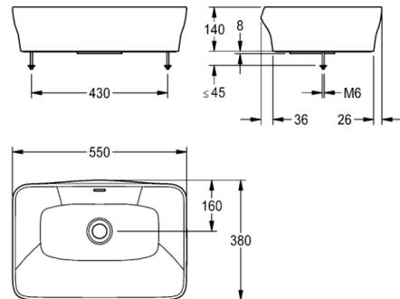
QUADROtop countertop basin, made of MIRANIT resin-bonded mineral material with pore-free, alpine white smooth surface (temperature-resistant up to 80 °C). Rectangular shape with rounded edges and seamless bowl, with overflow. No silicone sealant is required due to the invisible seal which is integrated in to the mounting edge. Drilling templates and mounting materials included.
