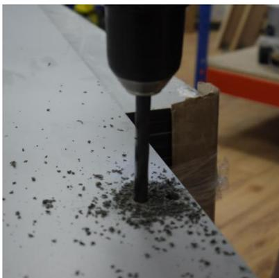
Work up through the drill bits to the required size required for the leg fixings.
