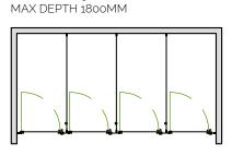
5 BETWEEN WALLS MAX WIDTH 4500MM MAX DEPTH 1800MM
